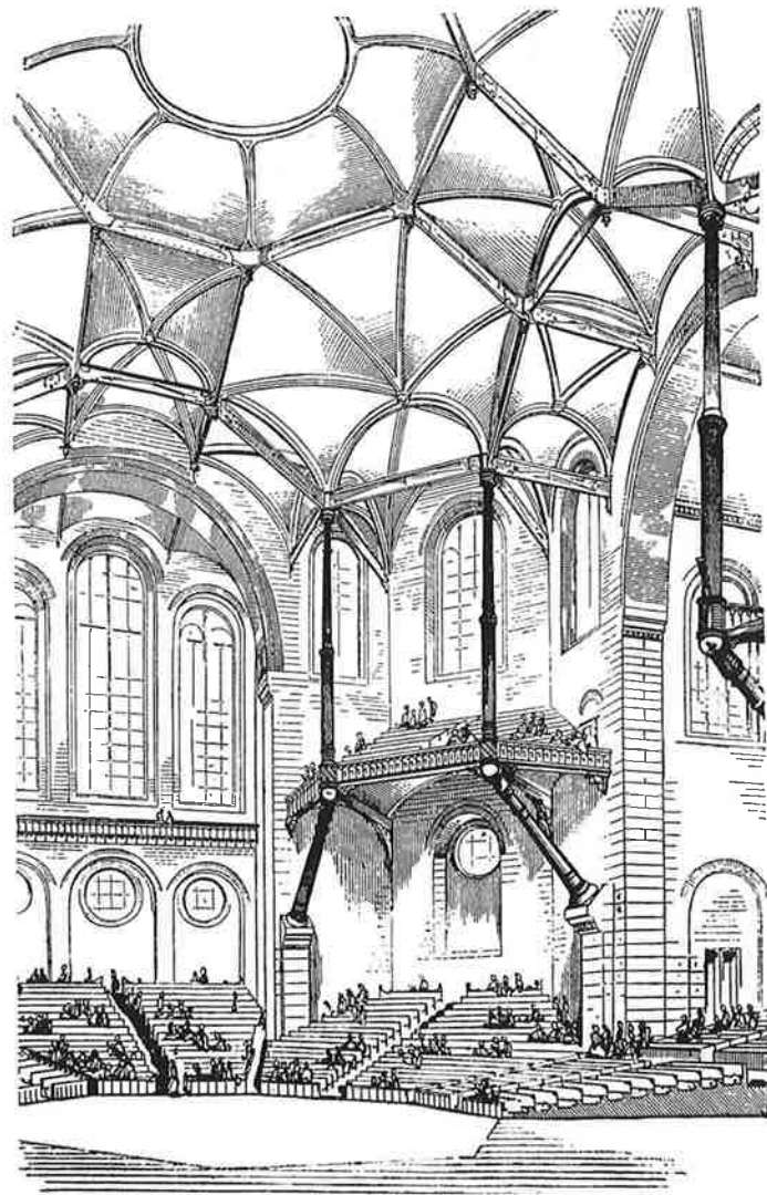
12-4 E.-E. Viollet-le-Duc. Concert hall for 3,000 with new method of vaulting. (From his Discourses on Architecture , Vol. II, 1863-72)
