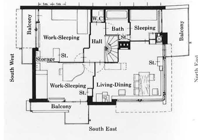
12-70 Second-story plan, with partitions extended, Schroeder House
