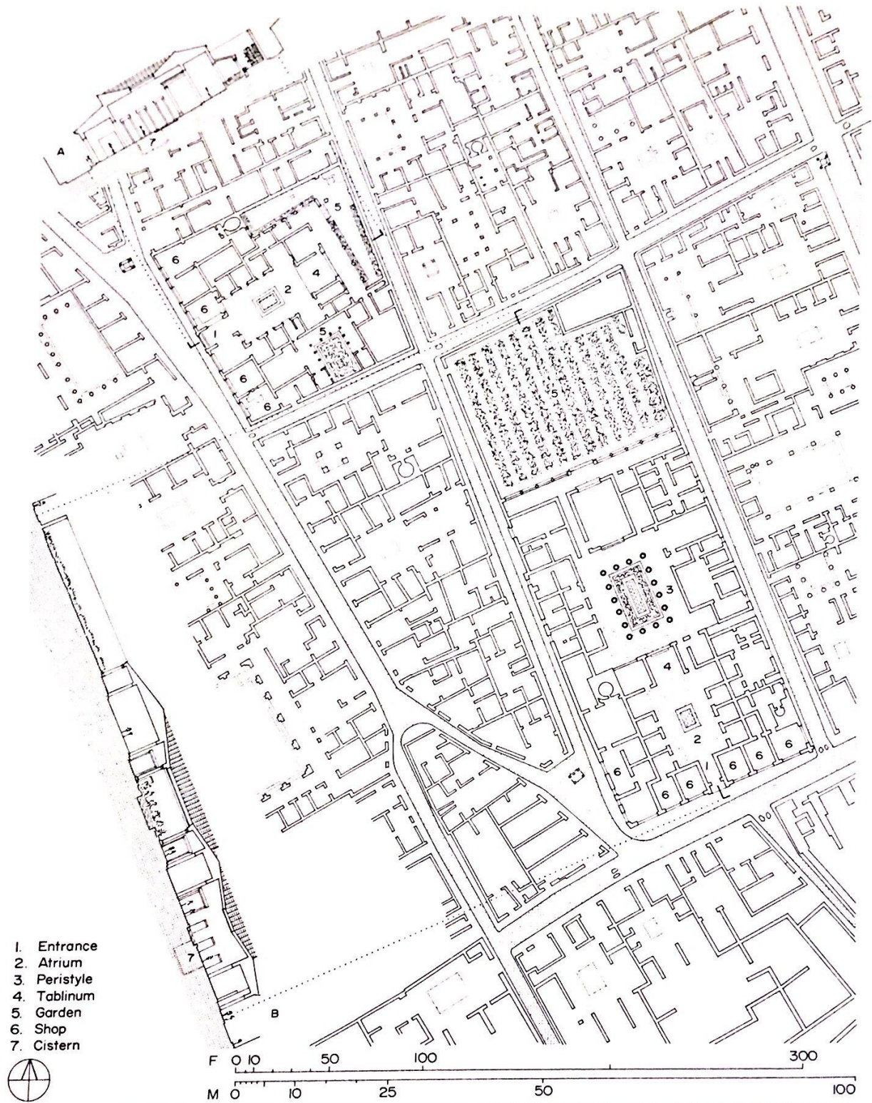
Fig. 9.9 Pompeii, residential neighborhood northwest of the Forum; plan. Two houses are highlighted: upper left, the House of Sallust, with a section through it shown at (A); and, lower left, the House of Pansa, with its section at (B). The House of Sallust dates from the pre-Roman
