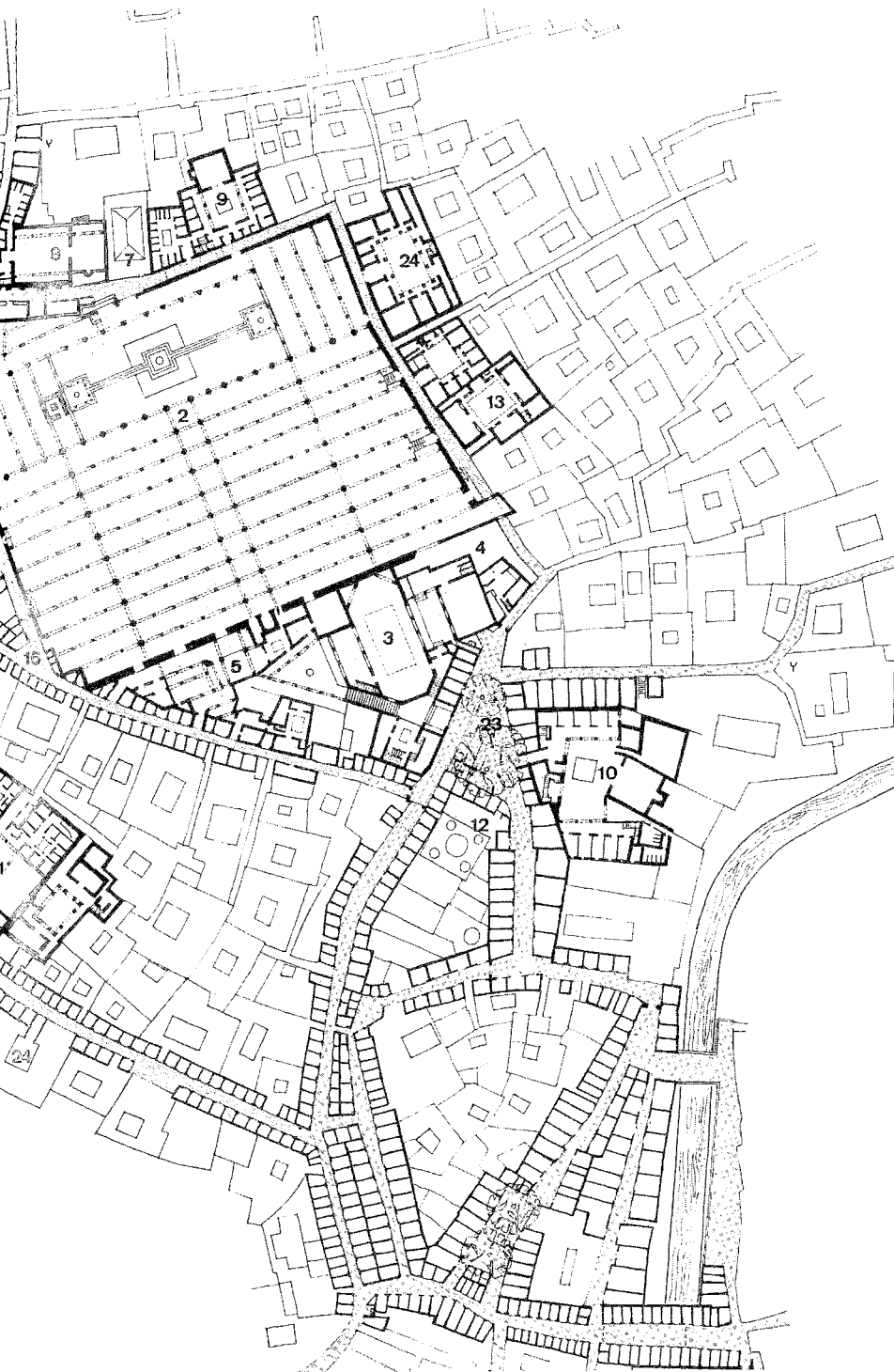
142 Plan of the traditional city centre of Fez al-Bali, showing the close interrelation existing between mosques, madrasas, suqs, caravanserais and residential districts.
