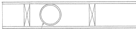
6" (150) stud wall • 5" (125) \varnothing hubless cast iron or plastic pipe • 3" (75) \varnothing bell-and-spigot cast iron pipe
