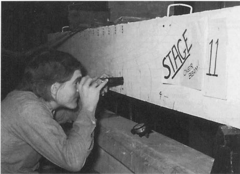
Photo 5.2 Simply supported beam prior to developing diagonal tension crack in flexure shear (load stage 11). (Test by Nawy et al.)
