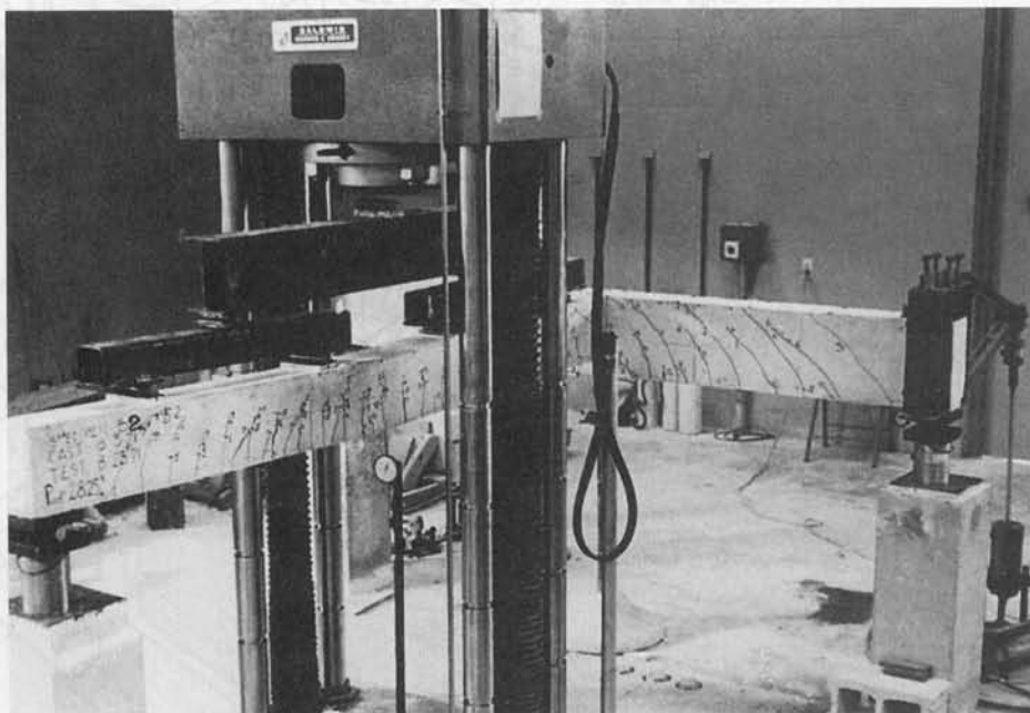
Photo 5.9 Reinforced concrete beams in torsion, testing setup. (Courtesy, Thomas T. C. Hsu.)
