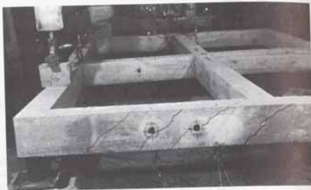
Inclined cracks due to torsion; test by J. P. Klus at the University of Wisconsin, Madison.
