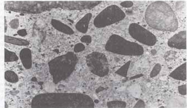
Figure 1.3.1 Cross-section of concrete. Cement and water paste completely coats each aggregate particle and fills all space between particles.
