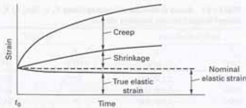
Figure 1.10.1 Change in strain of a loaded and drying specimen; t_0 is the time of application of load.
