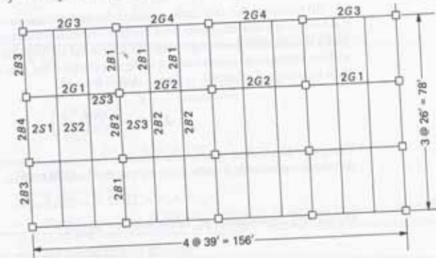
Figure 19.4.1 Floor plan of typical slab-beam-girder construction.
