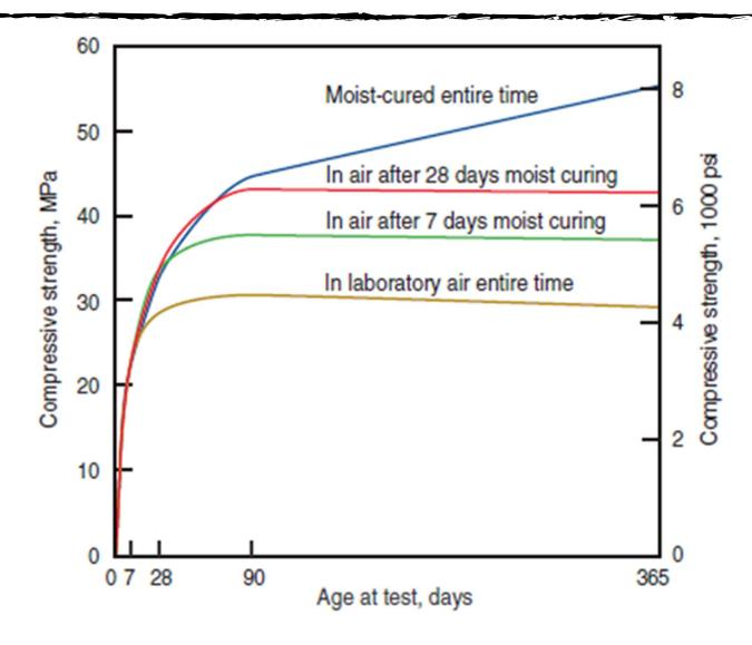
Effect of moist curing time on strength gain of concrete
