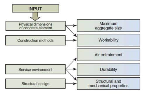
Durability is usually determined by the applicable specifications that lay down limiting values for a range of properties that must be satisfied. These properties are usually: the maximum water/cement ratio, minimum cement content, minimum strength, and air content for specific application or environment.
