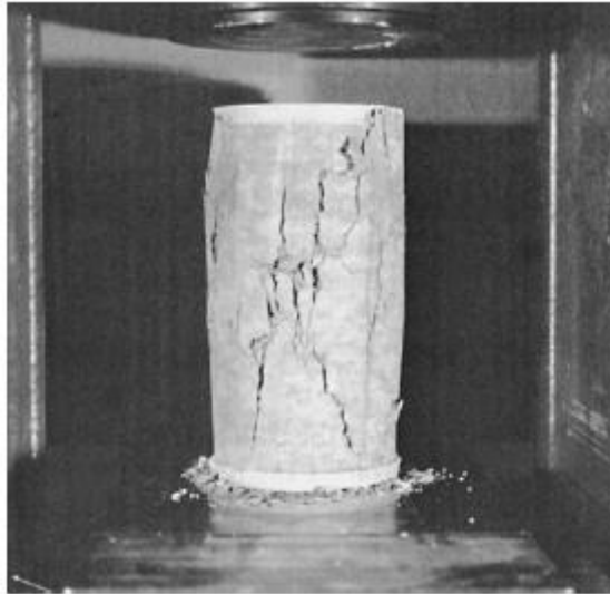
Figure 2-9: Typical failure mode of concrete in compression.
