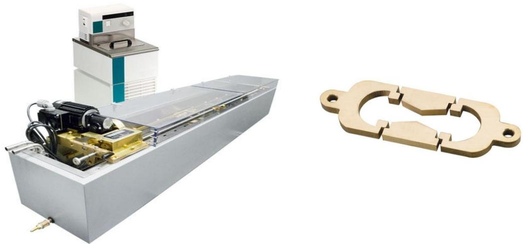
Figure 4 ductility test specimen and the mould
