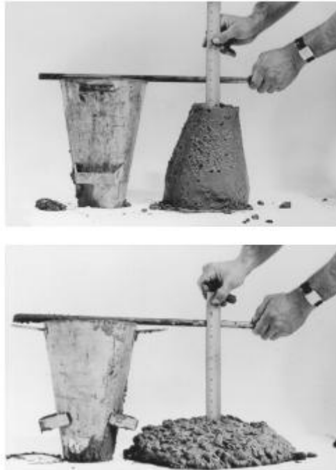
Figure 2-3: Demonstration on use of a slump cone: (top) a low slump and (bottom) a high slump.
