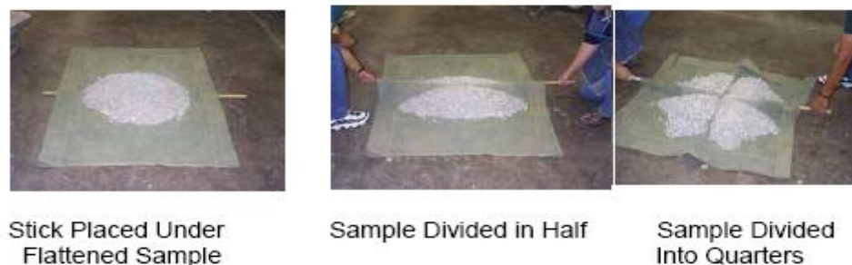
Figure 1-4: Alternative to B method
