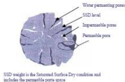
Fig.1-11: Diagram of Bulk SSD specific gravity
