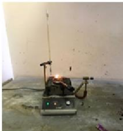
fig(1): fire and flash point settings
