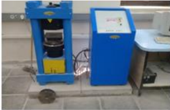
fig(3): compressive machine
