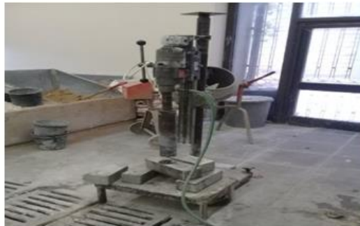
fig(6): core cutting drill
