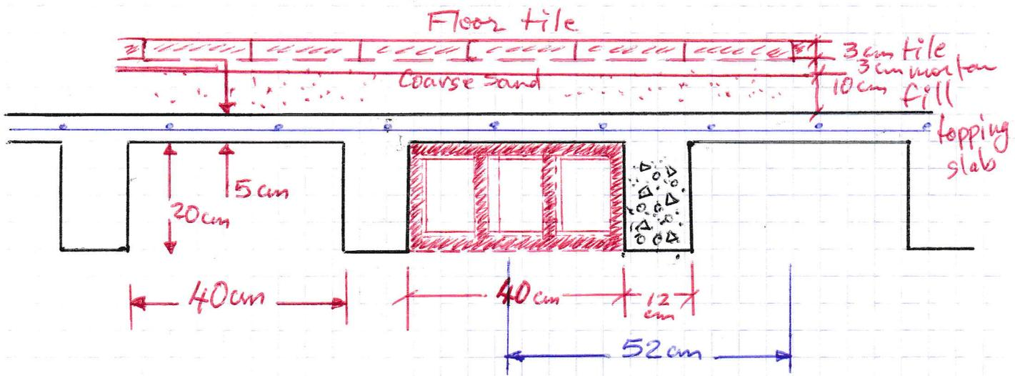
Live Load =  $150 \text{ kg/m}^2 (0.52) = 78 \text{ kg/linear m of rib}$
