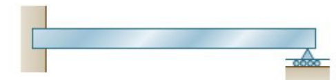
Beam fixed at one end and simply supported at the other end
