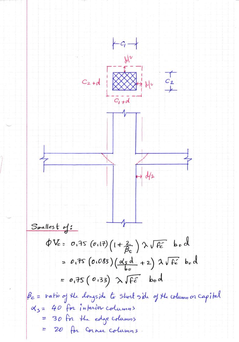
FIGURE 13.21 Failure surface defined by punching shear.
