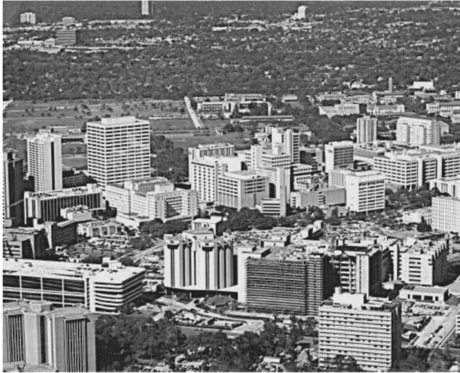
FIGURE C26.7-5(c) Exposure B: Structures in the Foreground Are Located in Exposure B. Structures in the Center Top of the Photograph Adjacent to the Clearing to the Left, Which Is Greater Than Approximately 656 ft (200 m) in Length, are Located in Exposure C When Wind Comes from the Left over the Clearing. (See Figure C26.7-4)
