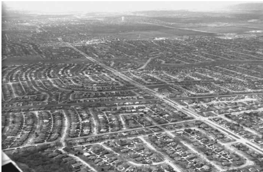
FIGURE C26.7-5(a) Exposure B: Suburban Residential Area with Mostly Single-Family Dwellings. Low-Rise Structures, Less Than 30 ft (9.1 m) High, in the Center of the Photograph Have Sites Designated as Exposure B with Surface Roughness Category B Terrain around the Site for a Distance Greater Than 1,500 ft (457 m) in Any Wind Direction
