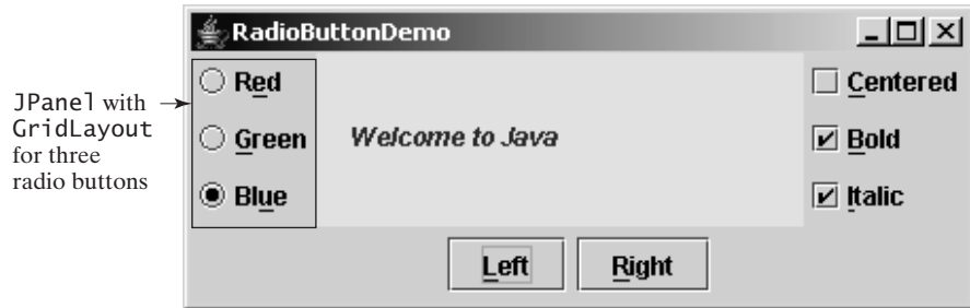
FIGURE 17.14 Three radio buttons are added to specify the color of the message.
