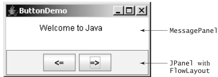
FIGURE 17.9 Clicking the <= and => buttons causes the message on the panel to move to the left and right, respectively.
