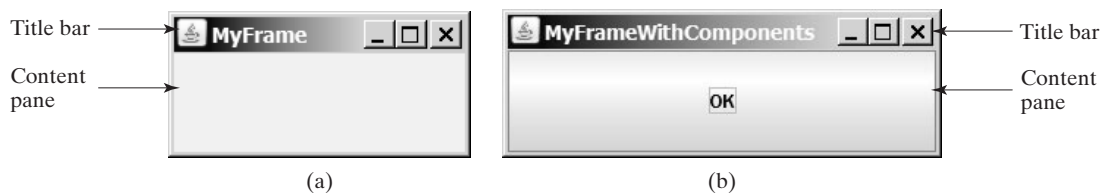
FIGURE 12.3 (a) The program creates and displays a frame with the title MyFrame . (b) An OK button is added to the frame.
