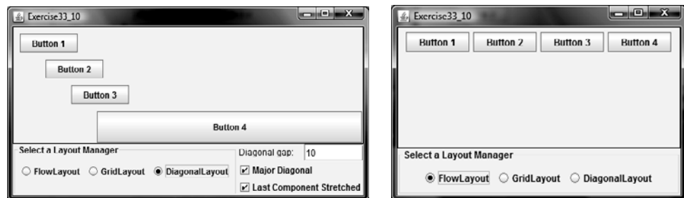
FIGURE 33.28 The program enables you to set the properties of the DiagonalLayout dynamically.
