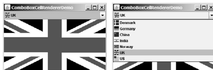
FIGURE 35.27 The image and the text are displayed in the list cell of a combo box.
