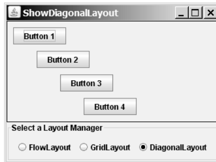
FIGURE 33.8 The DiagonalLayout manager places the components in a diagonal in the container.
