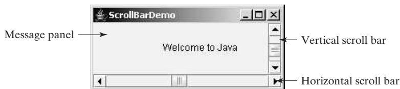
FIGURE 17.12 The scroll bars move the message on a panel horizontally and vertically.
