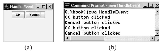
FIGURE 16.2 (a) The program displays two buttons. (b) A message is displayed in the console when a button is clicked.
