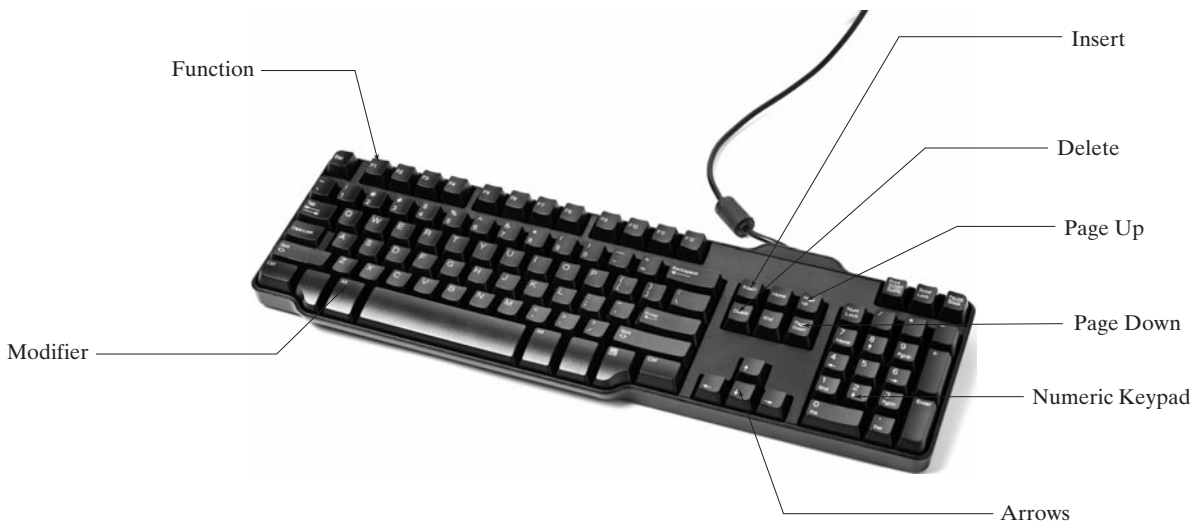
FIGURE 1.6 A computer keyboard consists of the keys for sending input to a computer.
