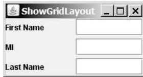
FIGURE 12.7 The GridLayout manager divides the container into grids; then the components are added to fill in the cells row by row.
