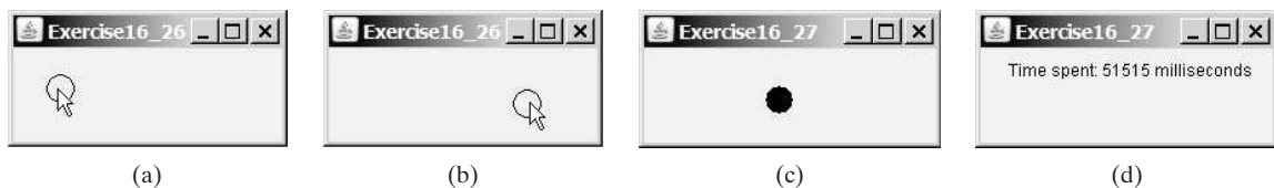
FIGURE 16.28 (a–b) You can point, drag, and move the circle. (c) When you click a circle, a new circle is displayed at a random location. (d) After 20 circles are clicked, the time spent is displayed in the panel.
