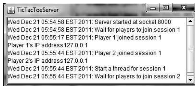
FIGURE 33.16 TicTacToeServer accepts connection requests and creates sessions to serve pairs of players.
