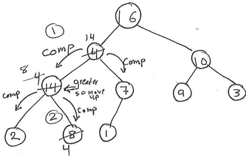
this is not a max heap, node with key 4 violates the max heap property.
