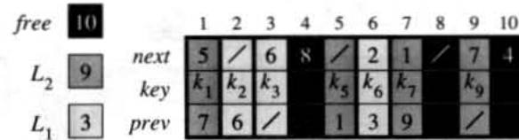
Figure 11.8 Two linked lists, L_1 (lightly shaded) and L_2 (heavily shaded), and a free list (darkened) intertwined.
