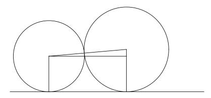
To place circle j, we compute where it would be placed if it were tangent to each of the first j-1 circles, selecting the maximum value. If this value is less than  $r_j$ , then we place circle j at  $x_j$ . The running time is  $O(N^2)$ .
