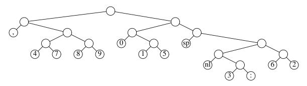
10.4 One method is to generate code that can be evaluated by a stack machine. The two operations are *Push* (the one node tree corresponding to) a symbol onto a stack and *Combine*, which pops two trees off the stack, merges them, and pushes the result back on. For the example in the text, the stack instructions are *Push(s)*, *Push(nl)*, *Combine*, *Push(t)*, *Combine*, *Push(a)*, *Combine*, *Push(e)*, *Combine*, *Push(i)*, *Push(s)*, *Combine*, *Combine*.
