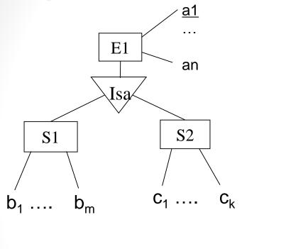
Method 1:  $E = (\underline{a}_{\underline{1}}, ..., a_{n})$   $S1 = (\underline{a}_{\underline{1}}, b_{1}, ..., b_{m})$   $S2 = (\underline{a}_{\underline{1}}, c_{1} ..., c_{k})$ Method 2:  $S1 = (\underline{a}_{\underline{1}}, ..., a_{n}, b_{1}, ..., b_{m})$  $S2 = (\underline{a}_{\underline{1}}, ..., a_{n}, c_{1} ..., c_{k})$
