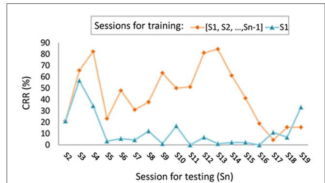
FIGURE 2 | Longitudinal variations in correct recognition rate (CRR) using two-stage person identification system with/without incremental learning, depicted by orange diamonds and blue triangles, respectively (figure depicted according to the results of self-paced finger movement experiment presented in our previous work, Cheng, 2013).
