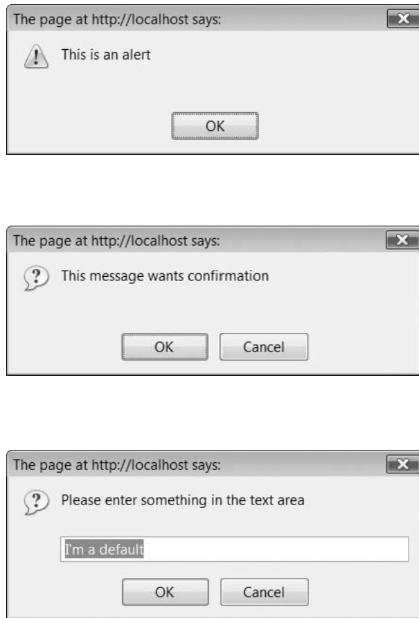
FIGURE 7.9 The three types of JavaScript dialog as they appear in Mozilla Firefox 2
