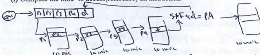
$$\text{Step} = 4 \Rightarrow \text{memory needed} = \text{step} + 1 = 5 \Rightarrow$$
