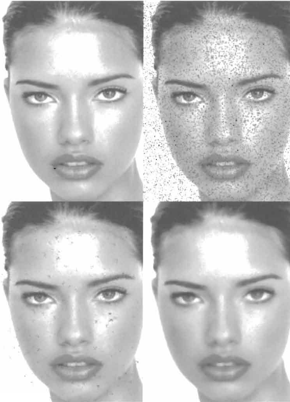
FIGURE 10 Impulse noise cleaning with a 5 \times 5 CWM smoother: (a) original "portrait" image, (b) image with salt- and-pepper noise, (c) CWM smoother with W_c = 16 , (d) CWM smoother with W_c = 5 . (See color section, p. C-3.)
