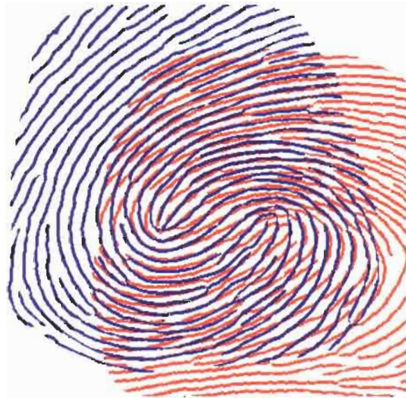
FIGURE 10.5.13 Aligned ridge structures of mated pairs. Note that the best alignment in one part (midleft) of the image results in a large displacements between the corresponding minutiae in the other regions (bottom right). © IEEE.
