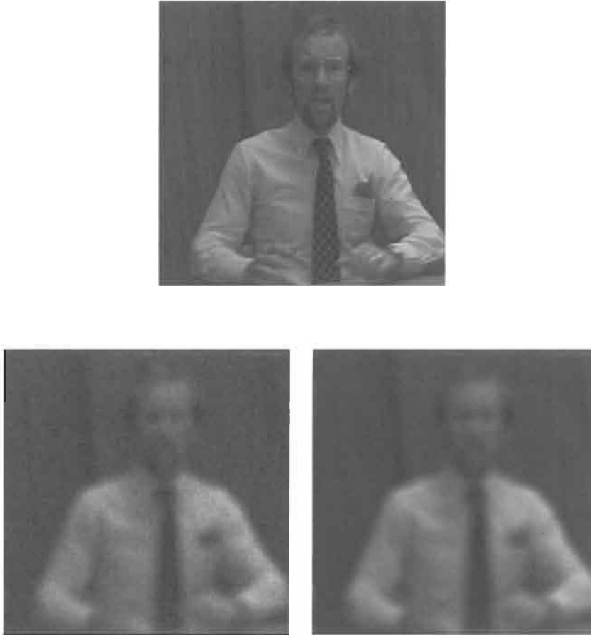
FIGURE 5 Original Image twy048 (top). Experiment I case (i) (bottom left): degraded image, with 11 \times 11 blur and 10 dB of BSNR additive noise. Experiment I case (ii) (bottom right): degraded image, with 11 \times 11 blur and 30 dB of BSNR additive noise.
