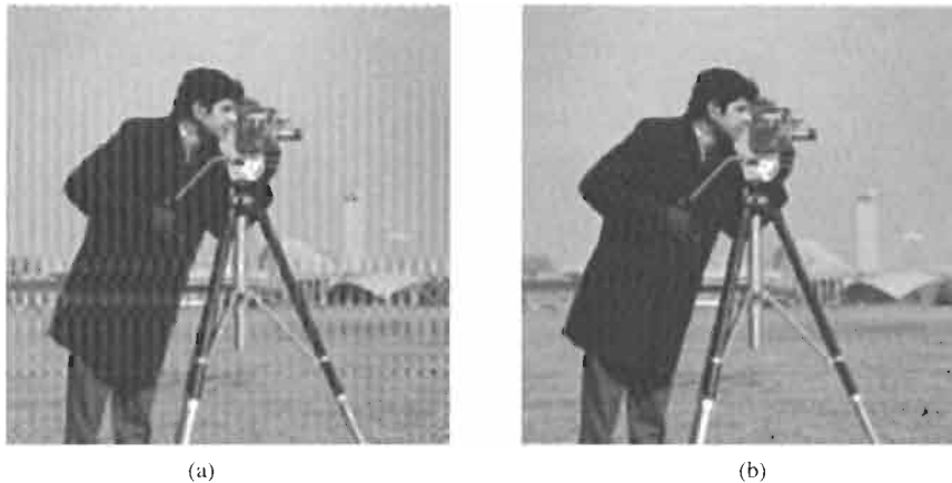
FIGURE 10 (a) Restored image illustrating the effect of the boundary value problem. The image was blurred by the motion blur shown in Fig. 2(a) and restored by using the constrained least-squares filter. (b) Preprocessed blurred image at its borders such that the boundary value problem is solved.
