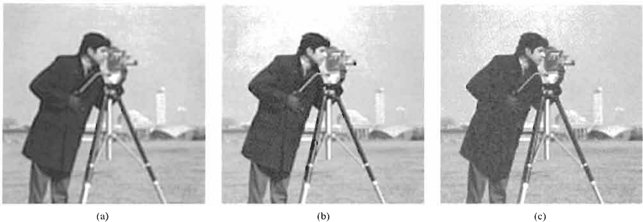
FIGURE 8 (a) Constrained least-squares restoration of image in Fig. 5(a) with \alpha = 2 \times 10^{-2} ( \Delta\text{SNR} = 1.7 dB), (b) \alpha = 2 \times 10^{-4} ( \Delta\text{SNR} = 6.9 dB), (c) \alpha = 2 \times 10^{-6} ( \Delta\text{SNR} = 0.8 dB).
