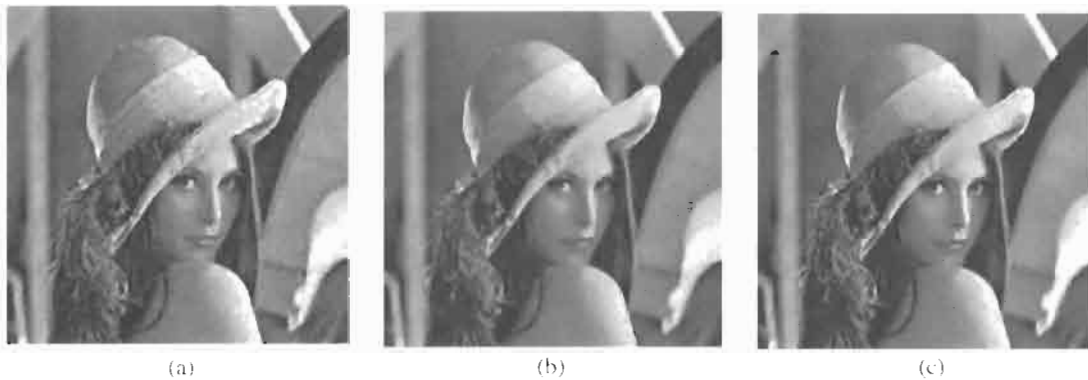
FIGURE 15 Dynamic coding of a still picture at a compression factor of 50:1. (a) Compressed by a linear subband decomposition; (b) compressed by a nonlinear subband decomposition; (c) compressed by dynamic coding that pits the two methods against each other.
