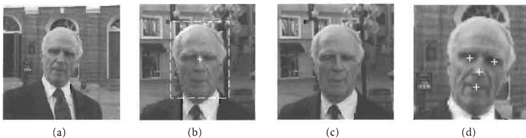
FIGURE 8 (a) Original image, (b) position and scale estimate, (c) normalized head image, (d) position of facial features.
