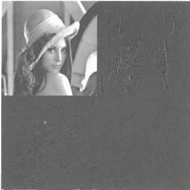
FIGURE 6 Decomposition of N \times M image into four N/2 \times M/2 subbands: (a) basic scheme, (b) application to Lena, using Daubechies' four-tap wavelet filters.
