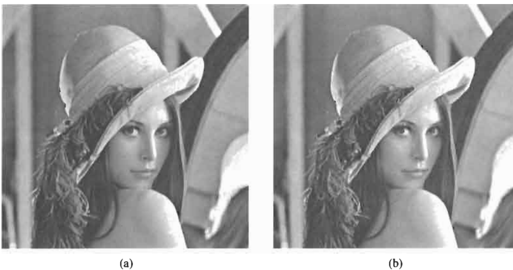
FIGURE 6 Perceptually lossless image compression [17]: (a) Original Lena image, 8 bpp; (b) decoded Lena image, 0.361 bpp. The perceptual thresholds are computed for a viewing distance equal to 6 times the image height.
