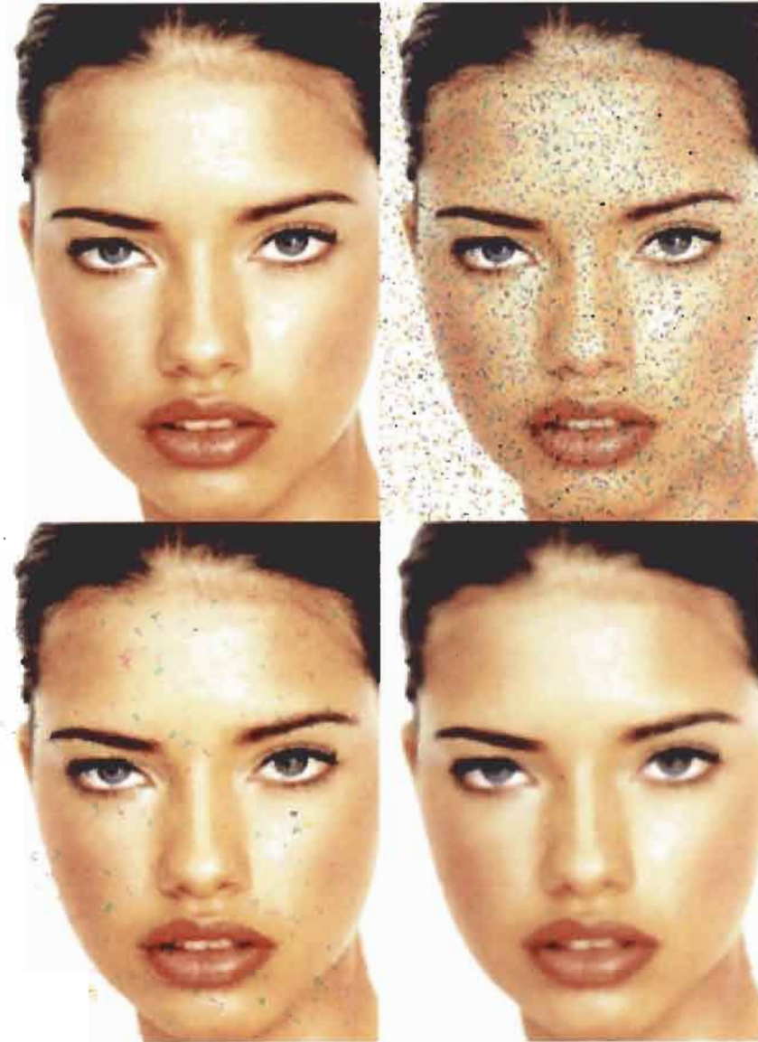
FIGURE 3.2.10 Impulse noise cleaning with a 5 \times 5 CWM smoother: (a) original “portrait” image, (b) image with salt- and-pepper noise, (c) CWM smoother with W_c = 16 , (d) CWM smoother with W_c = 5 .
