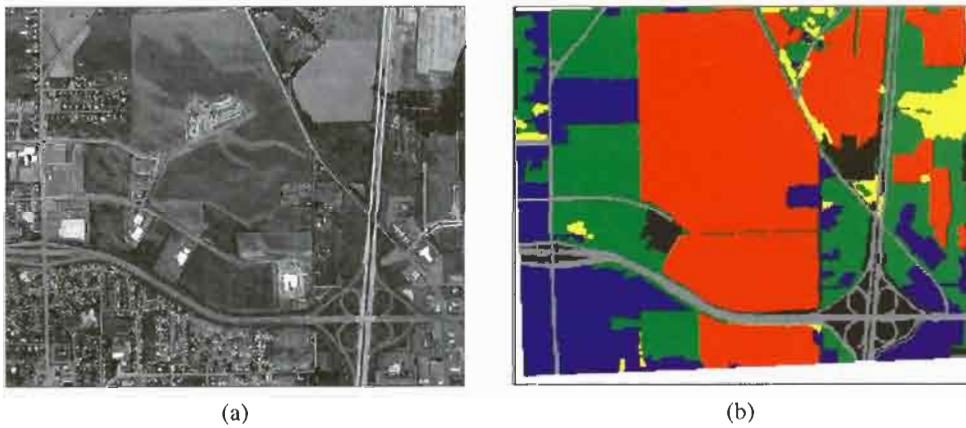
FIGURE 4.7.7 Updating old maps using image segmentation. (a) Aerial image of Eugene, Oregon in 1993. (b) Map of the same area in 1987. (c) Operator-assisted segmentation of the 1993 aerial image. (d) Updated map in 1993. ( Continued )
