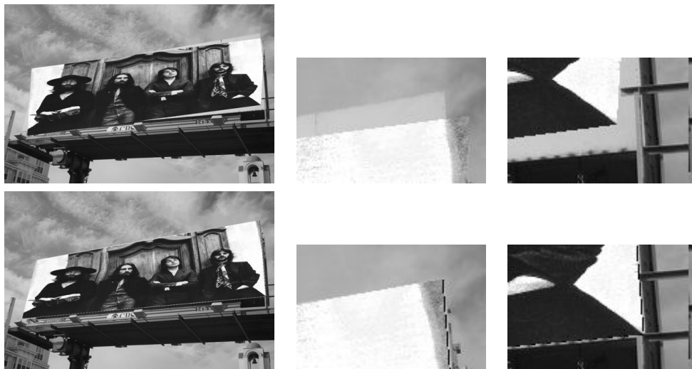
Figure 3.3: Comparing an affine warp of the full image with an affine warp using two triangles. The image is placed on a billboard with some perspective effects. (top) using an affine transform for the whole image results in a bad fit. The two right hand corners are enlarged for clarity. (bottom) using an affine warp consisting of two triangles gives an exact fit.
