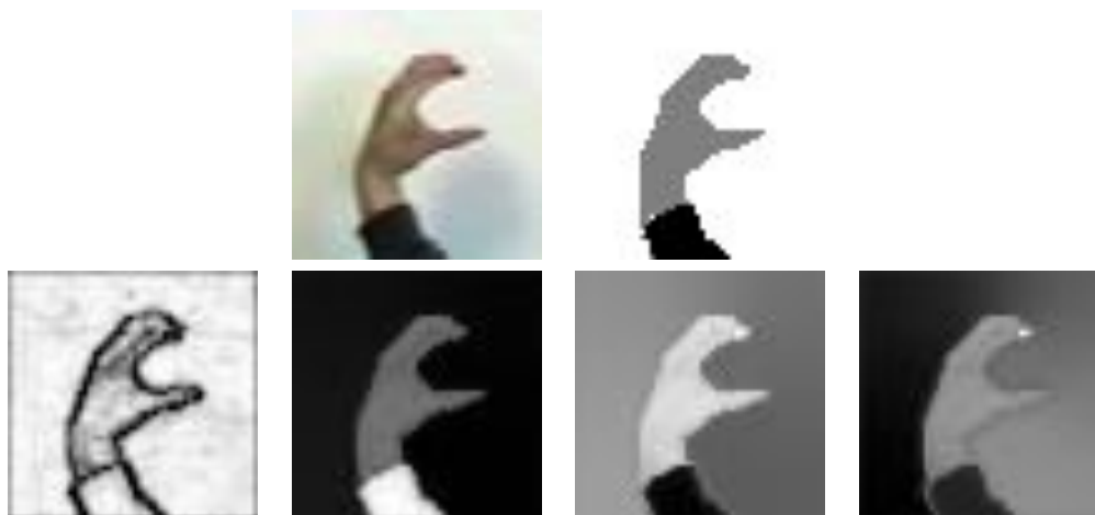
Figure 9.5: Image segmentation using the normalized cuts algorithm. (top) the original image and the resulting three-class segmentation. (bottom) the first four eigenvectors of the graph similarity matrix.
