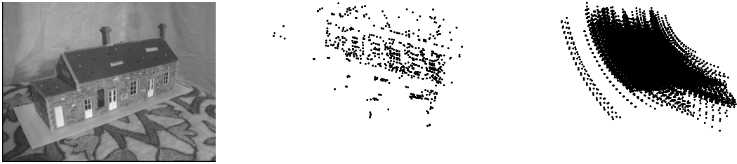
Figure 4.2: An example of projecting 3D points. (left) sample image. (middle) projected points into a view. (right) trajectory of projected points under camera rotation. Data from the Oxford "Model House" dataset.
