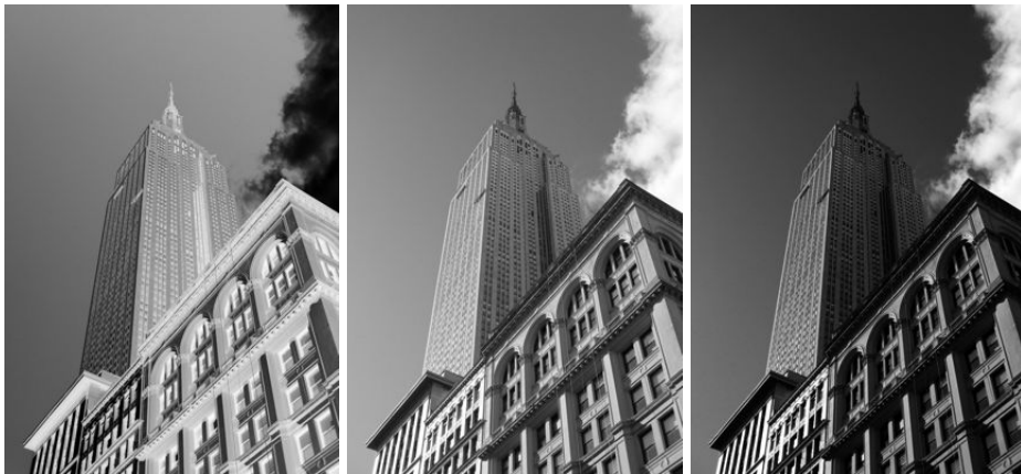
Figure 1.5: Graylevel transforms. Applying the functions in Figure 1.4. (left) Inverting the image with f(x) = 255 - x , (center) clamping the image with f(x) = (100/255)x + 100 , (right) quadratic transformation with f(x) = 255(x/255)^2 .
