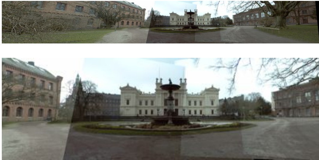
Figure 3.12: Horizontal panorama automatically created from SIFT correspondences. (top) the full panorama. (bottom) a crop of the central part.
