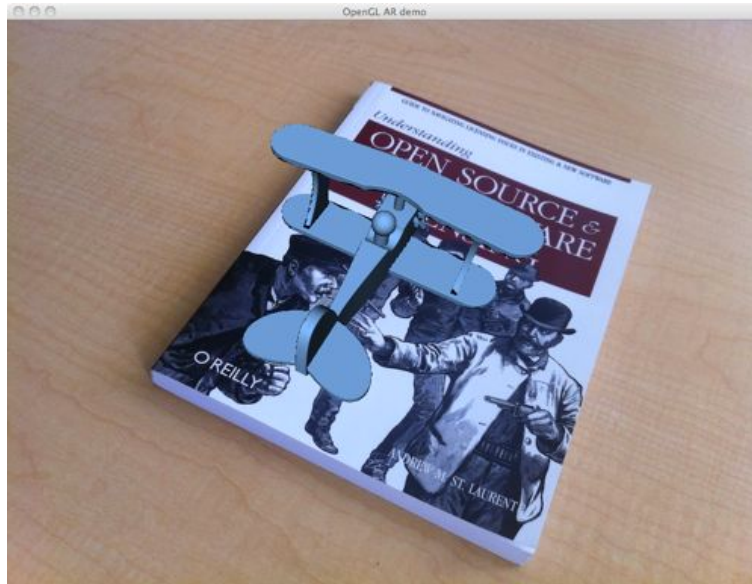
Figure 4.6: Loading a 3D model from an .obj file and placing it on a book in a scene using camera parameters computed from feature matches.
