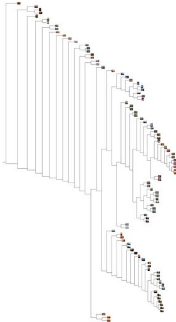
Figure 6.5: An example of hierarchical clustering of 100 images of sunsets using a 512 bin histogram in RGB coordinates as feature vector. Images close together in the tree have similar color distribution.
