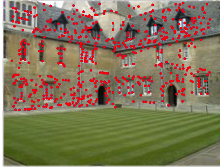
Figure 5.6: Projected points in view 1 computed using an estimated camera matrix.
