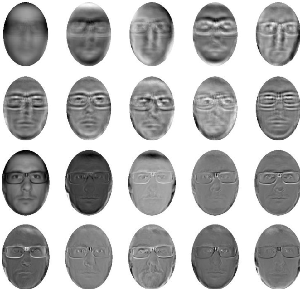
Figure 3.8: Comparing PCA-modes of unregistered and registered images. (top) the mean image and the first nine principal components without registering the images beforehand. (bottom) the same with the registered images.
