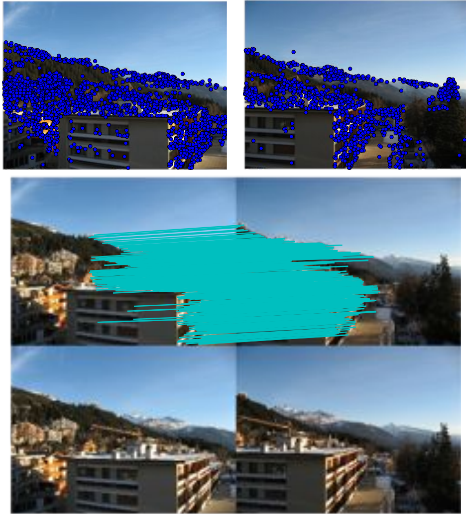
Figure 2.5: An example of detecting and matching SIFT features between two images.
