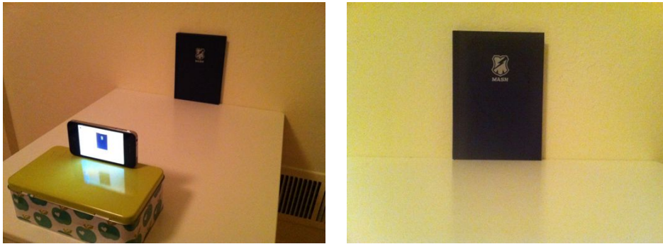
Figure 4.3: A simple camera calibration setup. (left) an image of the setup used. (right) the image used for the calibration. Measuring the width and height of the calibration object in the image and the physical dimensions of the setup is enough to determine the focal length.
