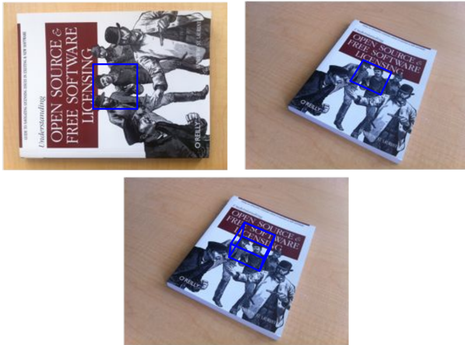
Figure 4.4: Example of computing the projection matrix for a new view using a planar object as marker. Matching image features to an aligned marker gives a homography that can be used to compute the pose of the camera. (top left) template image with a blue square. (top right) an image taken from an unknown viewpoint with the same square transformed with the estimated homography. (bottom) a cube transformed using the estimated camera matrix.
