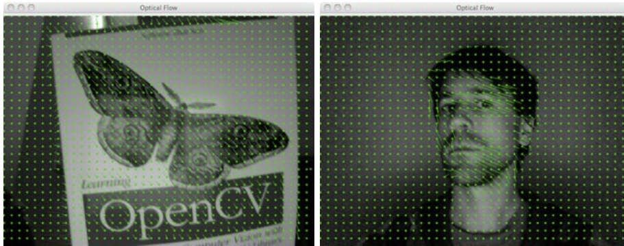
Figure 10.5: Optical flow vectors (sampled at every 16th pixel) shown on video of a translating book and a turning head.
