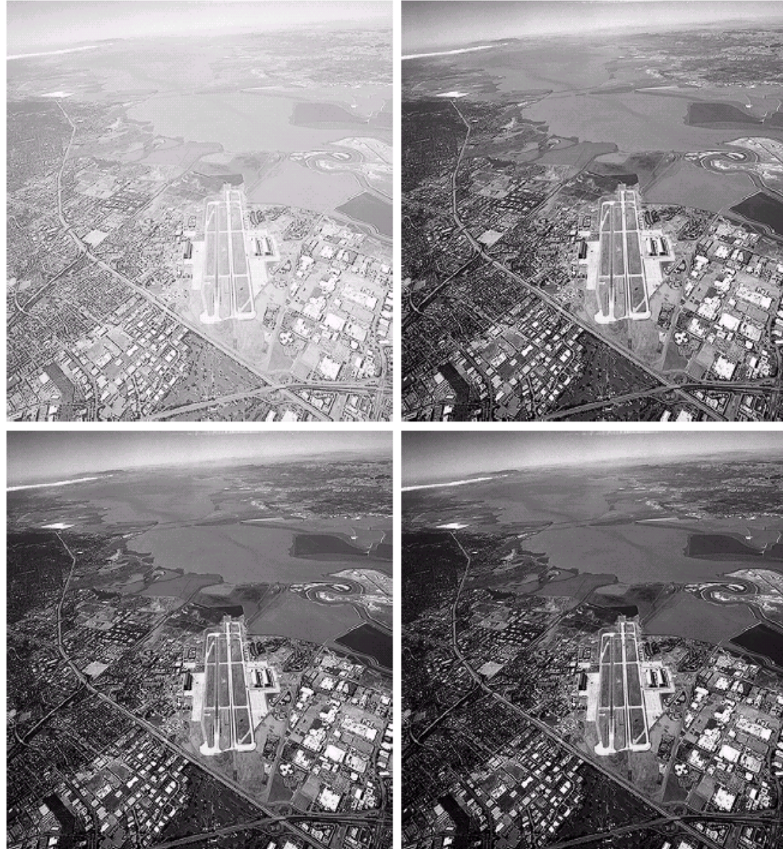
FIGURE 3.9 (a) Aerial image. (b)–(d) Results of applying the transformation in Eq. (3.2-3) with c = 1 and \gamma = 3.0, 4.0, and 5.0, respectively. (Original image for this example courtesy of NASA.)
