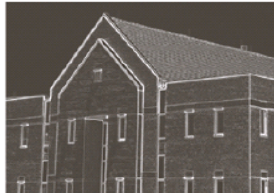
Gradient Image ( |G_x| + |G_y| ) after the original image was smoothed by 5x5 mask
