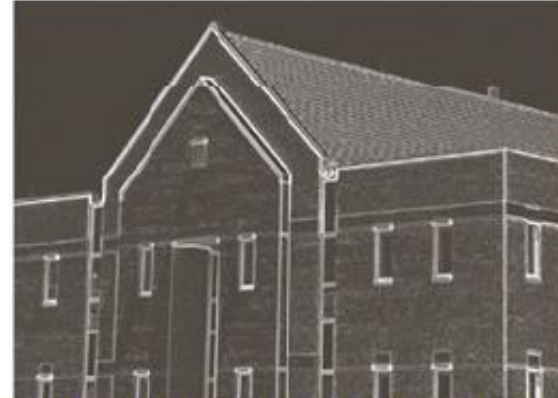
Gradient Image ( |G_x| + |G_y| ) after the original image was smoothed by 5x5 mask
