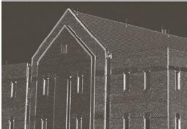
Gy computed using Sobel Operator
