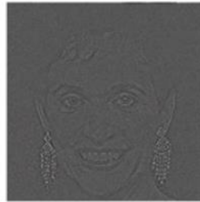
Image Reconstructed Using Phase only
