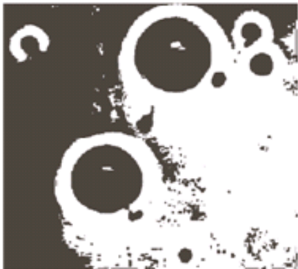
Segmentation using basic global thresholding T^* = 169
