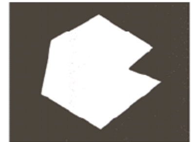
Segmentation result after applying Otsu's method to each subimage
