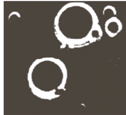
Segmentation using Otsu's global thresholding k^* = 181
