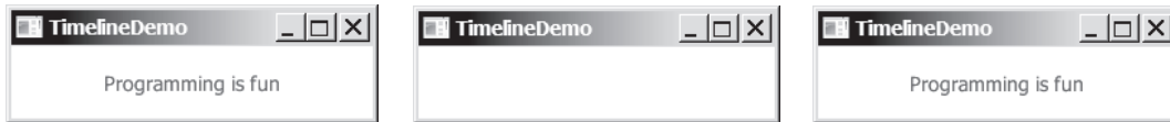
FIGURE 15.21 The handler is called to set the text to “Programming is fun” or empty in turn.
