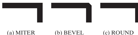
FIGURE 31.16 Path segments can be joined in three ways: (a) MITER, (b) BEVEL, and (c) ROUND.
