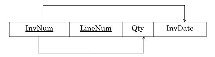
Candidate keys: {InvNum, LineNum} InvDate is *partially dependent* on {InvNum, LineNum} as InvNum is a determinant of InvDate and InvNum is part of a candidate key
