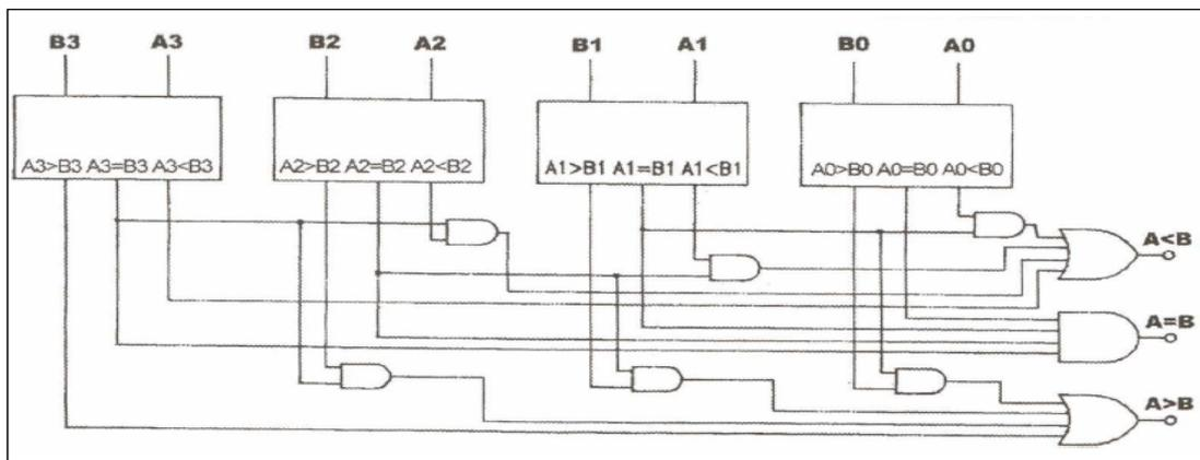
(a) Constructed with four 1-bit Comparators
