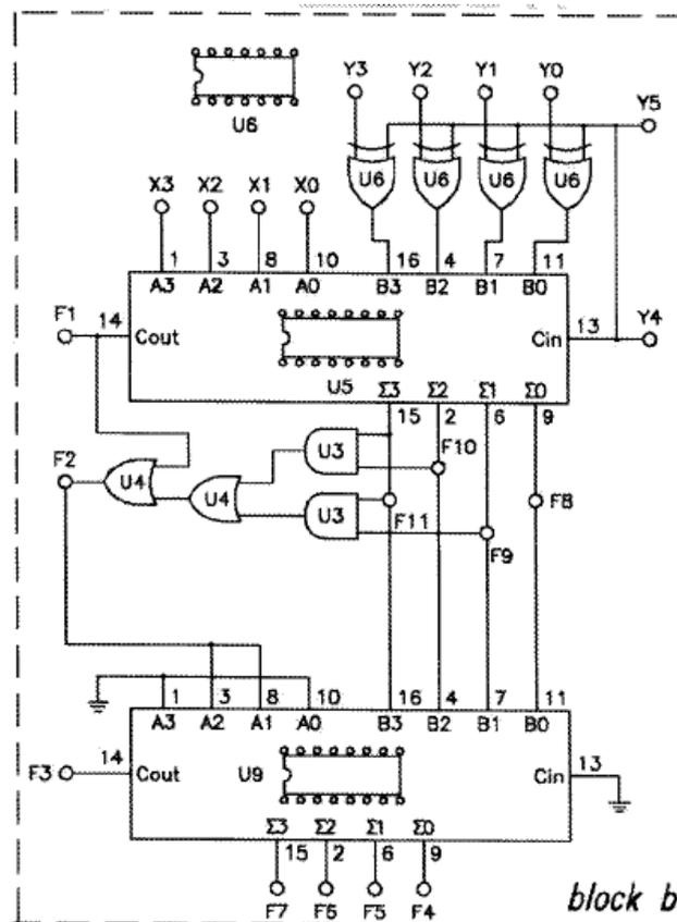
FIG1.11: Wiring Diagram (KL-26002 block b)
