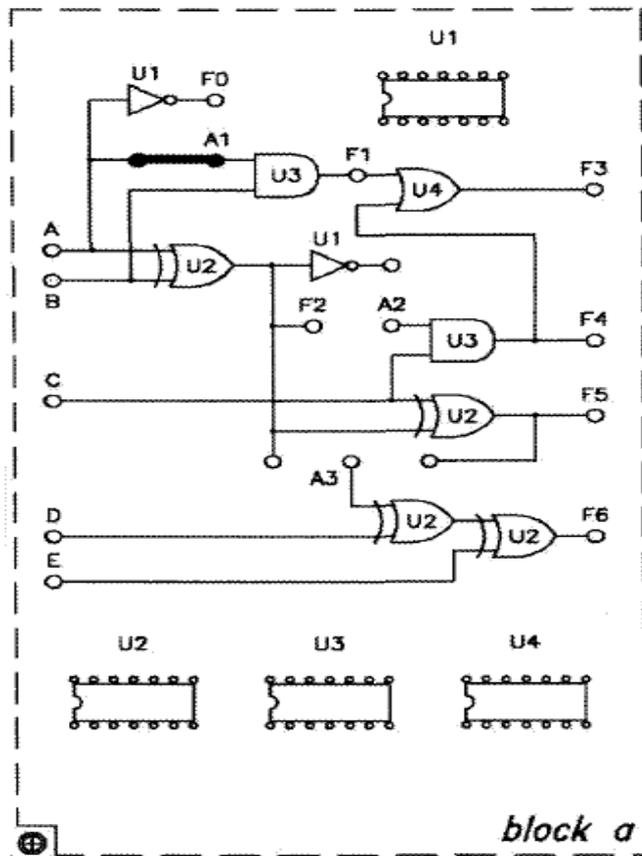
FIG1.7: Wiring Diagram (KL-26002 Block a)
