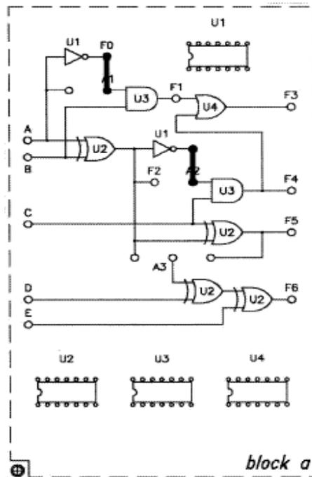
FIG1.13: Wiring Diagram (KL-26002 block a)
