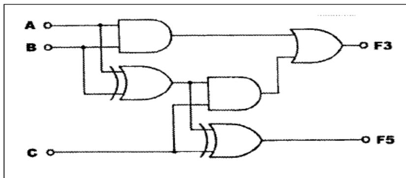
FIG1.9: Full-Adder Circuit
