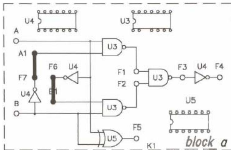
(a) Wiring diagram (KL-26001 block a)
