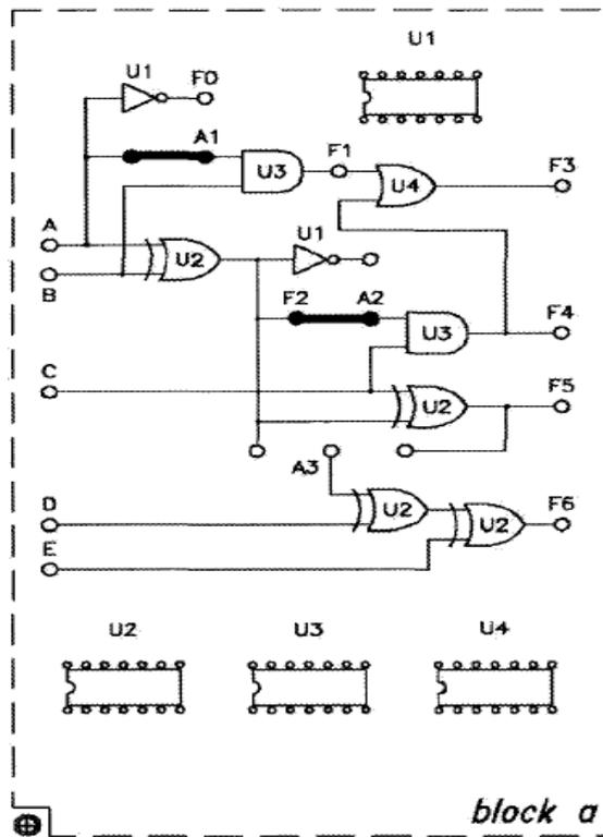
FIG1.10: Wiring Diagram (KL-26002 Block a)
