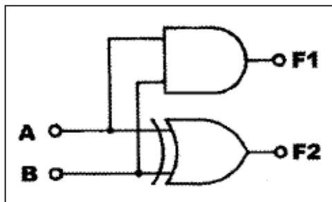
FIG1.8: Half-Adder Circuit
