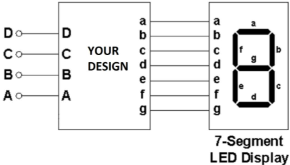
Your system will have 4 inputs (A, B, C, D) and 7 outputs (a through g) that drive a 7-segment display, whose inputs are active-high. The system shall behave according to the following table:
