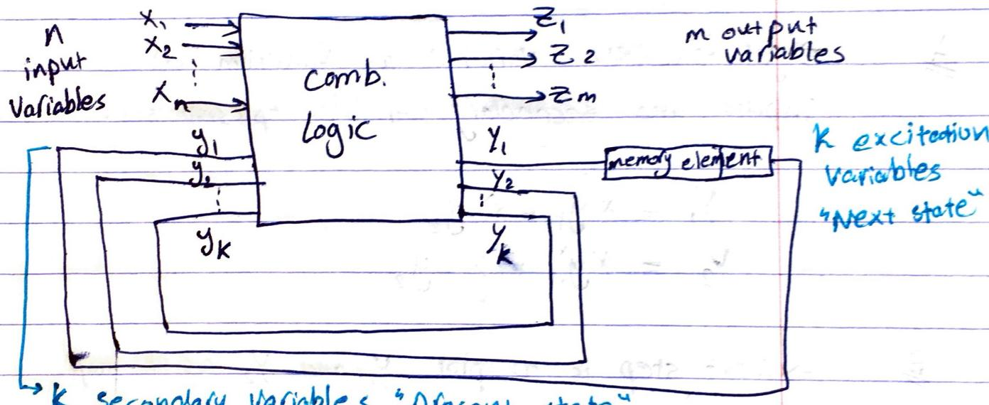
\* circuit is stable when  $y_i = y'_i$  for all  $i=1,2,\dots$
