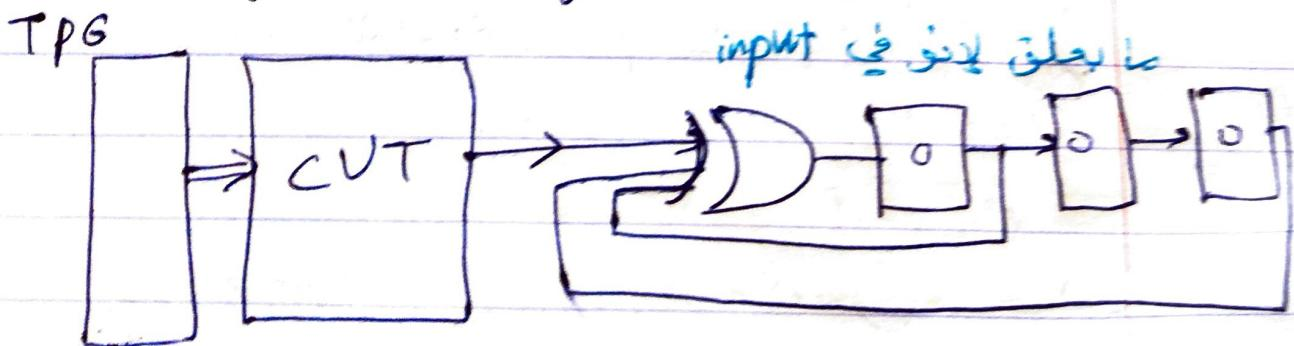
Ex: Signature analyzer is initialized to all zero state, this signature register is fed with data stream 10111 (LSB arrive first)
