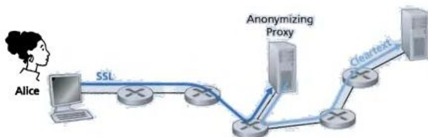
Figure 8.36 ♦ Providing anonymity and privacy with a proxy
