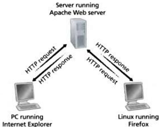
Figure 2.6 ♦ HTTP request-response behavior
