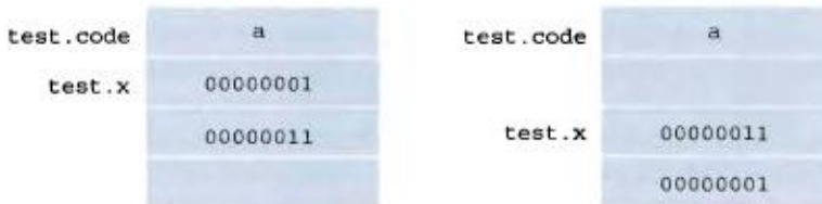
Figure 9.6 ♦ Two different data layouts on two different architectures
