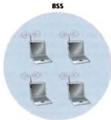
Figure 6.8 ♦ An IEEE 802.11 ad hoc network
