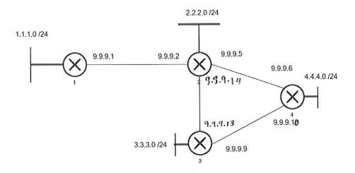
In the above diagram, write a minimal static routing policy (table) for each of the routers to make all networks accessible form everywhere.
