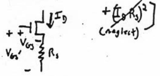
$$I_D \left[ 1 + K' \frac{W}{L} (V_{GS} - V_t) R_S \right] \\ = \frac{K'}{2} \frac{W}{L} (V_{GS} - V_t)^2$$
