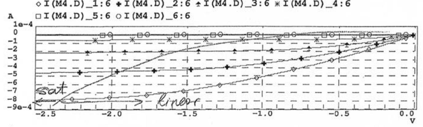
c) 1&3 are in velocity sat, The effect can be seen from the linearly increasing  $I_D$ .
