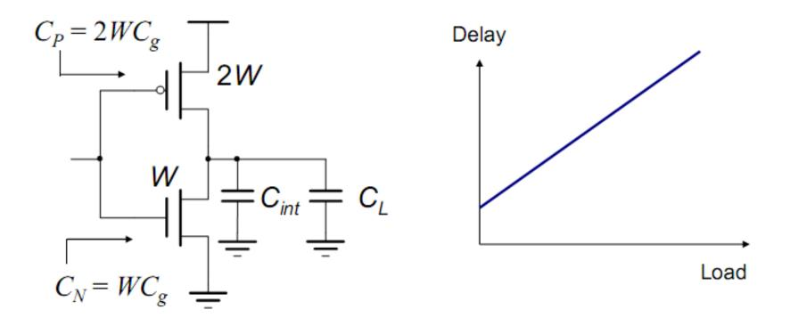
Delay =  $kR_W C_{in}(C_{int}/C_{in} + C_L/C_{in})$ =  $3kLR_{sq,n}C_g[C_d/C_g + C_L/(3WC_g)]$ = Delay (Internal) + Delay (Load)
