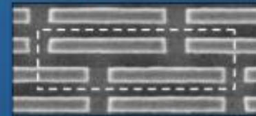
0.108 \mu\text{m}^2 SRAM cell for low voltage applications
