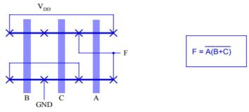
B. Implement the following circuit in stick diagram. Assume all inputs are given and do not break the diffusion. (4 pts)
