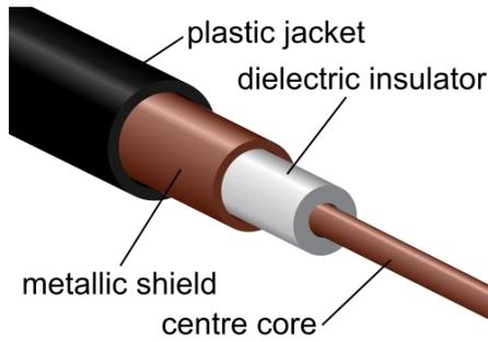
Figure 1-3 Coaxial cable
