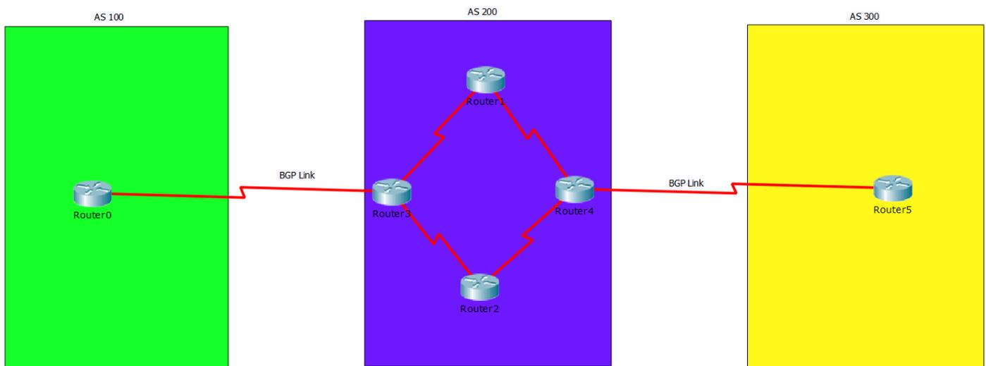
Figure 5-1 AS Connecting with BGP Links
