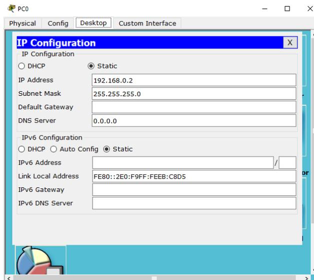
Figure 2-3 PC0 IP address
