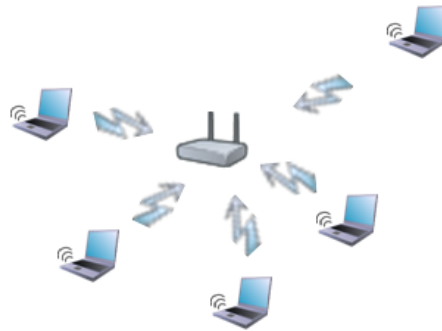
Figure 2: WLAN in Access Point Mode
