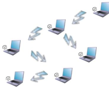
Figure 1: Ad Hoc WLAN
