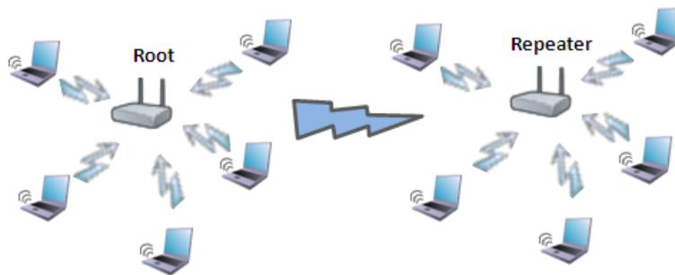
Figure 3: WLAN with Wireless Repeater
