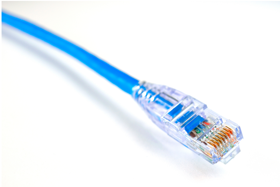
Figure 4: 8P8C modular connector, commonly referred to as RJ45, used for the Ethernet standard, reference [4].
