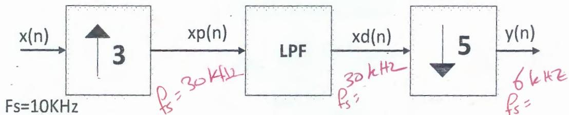
A speech signal sampled at 10KHz,  $x(n)$  has a spectrum magnitude  $|X(e^{j\omega})|$  as shown below, is applied to the above system. Assume LPF is an ideal Lowpass filter with magnitude of 1.
