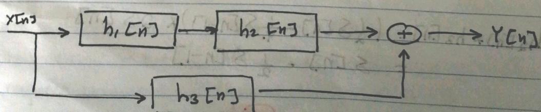
**Exercise:** Determine the overall impulse response of the following system, where the impulse responses of the components systems are:
