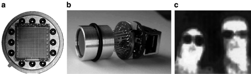
Fig. 14.21 Thermopile thermal-imaging sensor: sensing surface (a); imaging module (b); and example of a thermal image (c) (courtesy of Heimann Sensors, www.heimannsensor.com )
