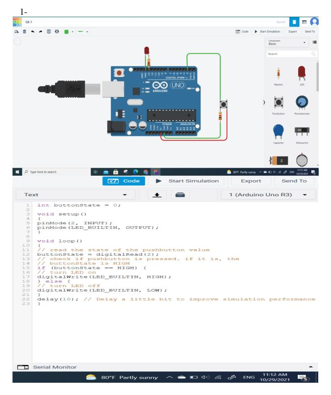
In this circuit push button used to turn on the LED and when we push it again the LED will turn off as representation for pullup/pulldown resistor.
