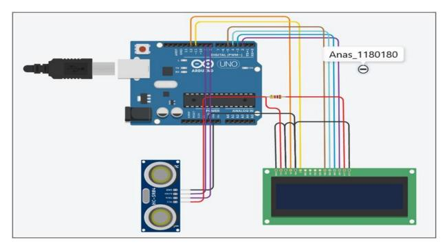
In this case the idea is the same as the previous requirement but instead of show the result on 7 segment chips the distance shown in cm on LCD as shown in the figures below: -
