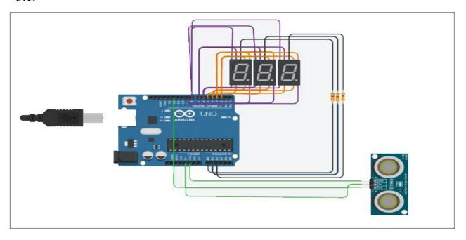
The figure shown an Arduino circuit which sense if there's a body in distance from 3cm to 336cm using ultrasonic distance sensor then this value shown on 7 segment chips the code in appendix includes the required comments where the figures below show the running process:
